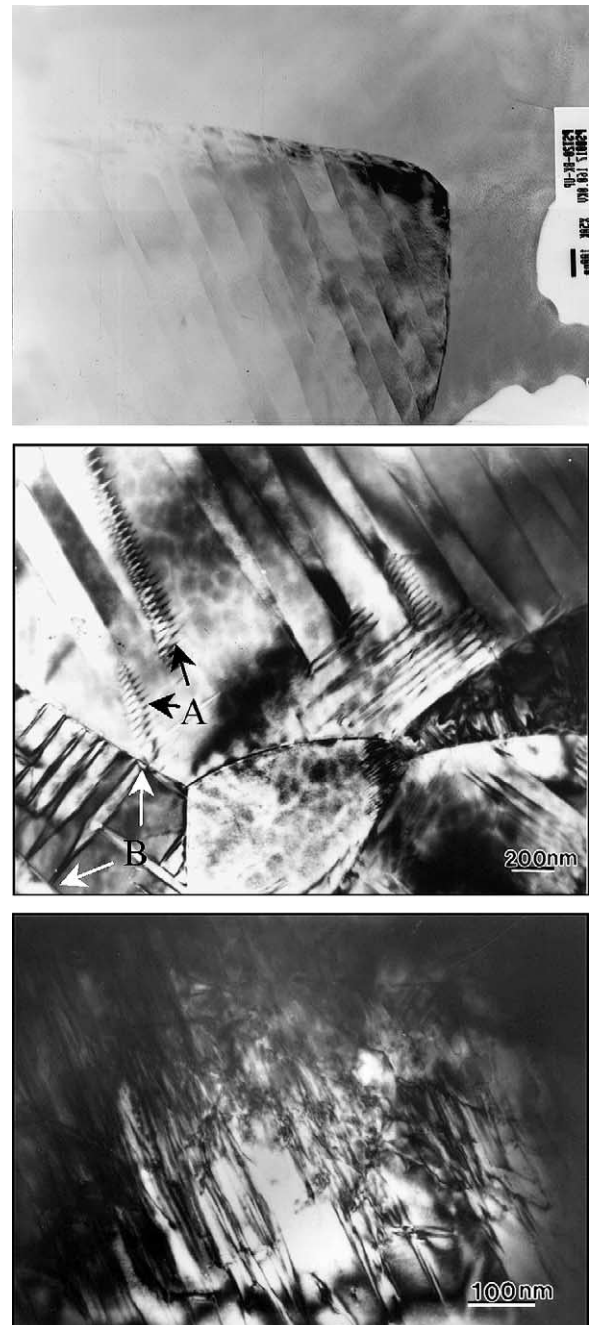
Fig. 2. TEM micrographs showing microstructural evolution of \text{Pb}_{0.6}\text{Sr}_{0.4}\text{TiO}_3 ceramics under polarization switching at a working frequency of 1 kHz and 55 kV/cm. (a) as-sintered state; (b) polarization switching for 10^5 cycles; (c) 3 \times 10^9 switching cycles.
